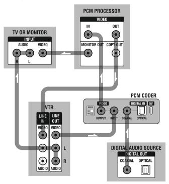
Connect the VIDEO OUT of the VTR jack to the VIDEO IN jack of the PCM Coder for PCM playback from a VTR on the PCM Processor. PCM Coder will pass-through signal to the PCM processor while the PCM coder in standby mode or power off.
