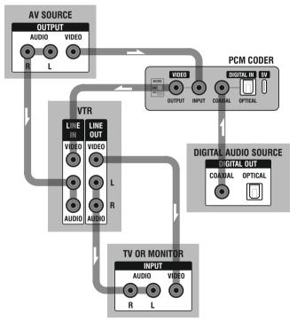
PCM Coder can pass-through video signal via VIDEO IN jack to the VIDEO OUT jack in standby mode or power off.
