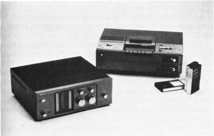
Fig. 4-14. B-Format (the first PCM recorder ever marketed. PCM-1 and a betamax VTR. Table 4-2 No. 7).
