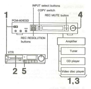
Set the switches below to the appropriate position or press the appropriate button.
