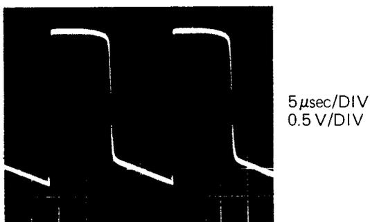
8. Turn RV103 (RV203) fully counterclockwise. The base of the waveform at TP103 (TP203) becomes doubly as shown below. This is called as 1st double base.
